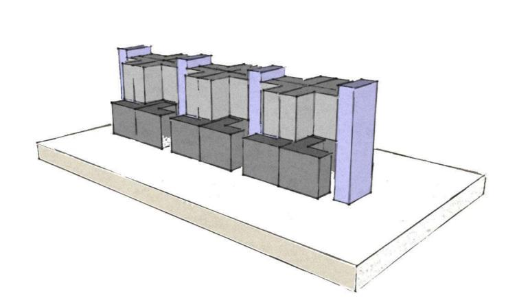
The larger intent is to try and be responsive to dwellings at different heights. In the process of achieving a configuration like this, the building is supported and accessed by the cores in the middle and the ends. The ground floor is left open on stilts. The 6th floor is a free floor which can act as a refuge space/ space for semi-open gatherings and small parties and also ventilates the cutouts below. From the 7th floor, the configuration changes.
