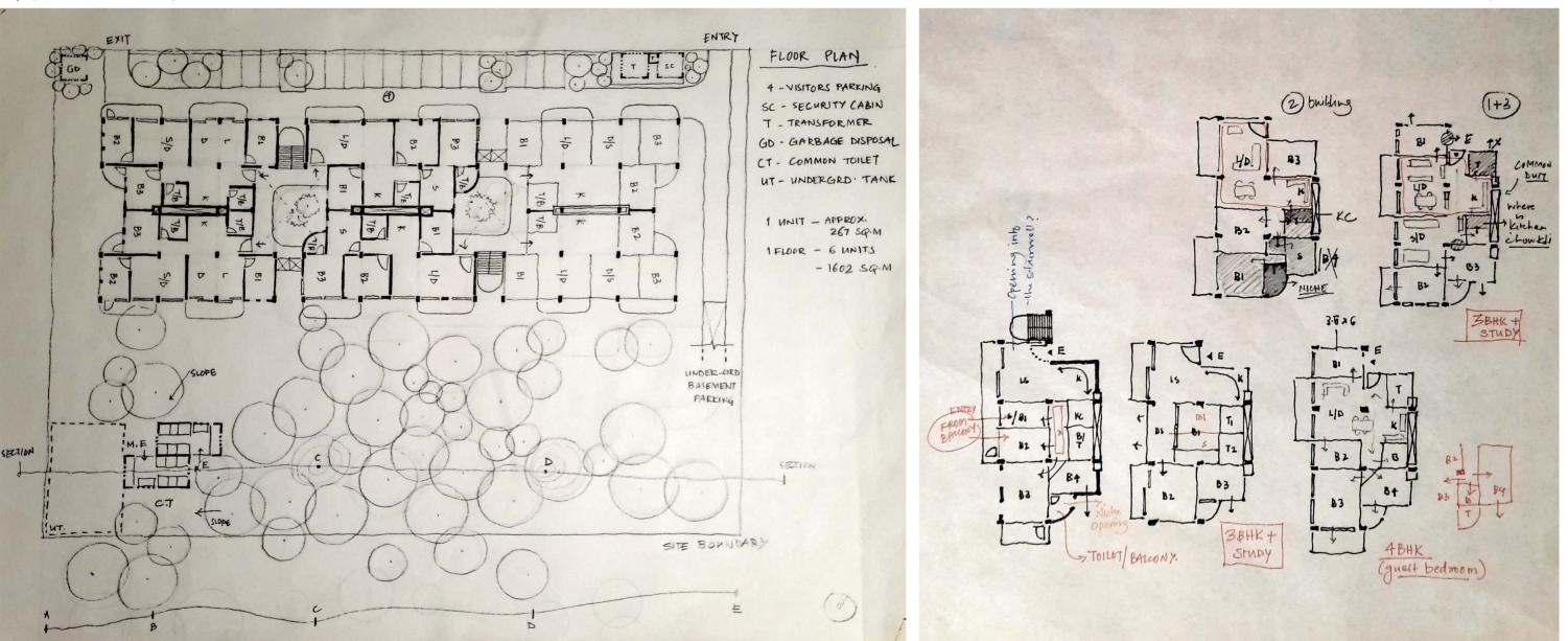
Plot area- 5850 sq.m | FSI- R2 zone 1.8 | Total Built up area- 10530 sq.m Ground cover- 1870 sq.m Type A/ Type B unit- Approx. 267 sq.m 1 Floor- 6 units- 1602 sq.m Total 6 floors- 18 m building height
